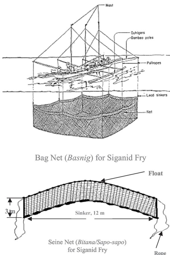
**Fig. 5** Bagnet and seine-net, the two fishing gears that catch siganid juveniles in Lagonoy Gulf.
